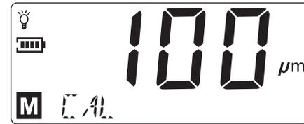
choose a standard piece, its thickness is at 95~105, press 'up' and 'down' key to amend the display value, make the display value accord with the standard piece's thickness, and then place the standard piece on the iron basic to adjust.
