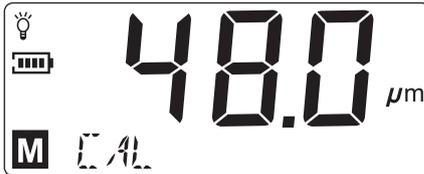
Choose a standard piece, its thickness is at 45~55, press UP and DOWN key to amend the display value, make the display value accord with the standard piece's thickness, and then place the standard piece on the iron basic to adjust.
