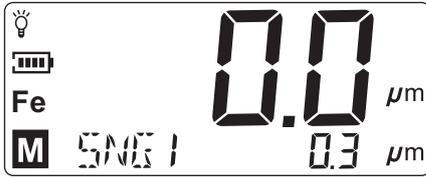
c. If you want to correctly adjusted, you must repeat a and b to make basic measure value less than 1μm, this can improve measurement precision.
